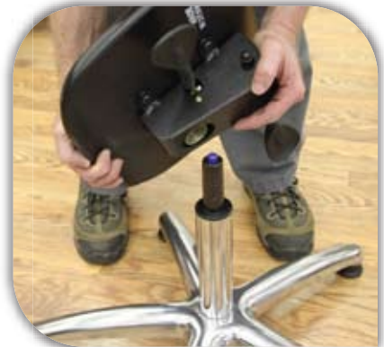
Insert seat onto cylinder shaft
