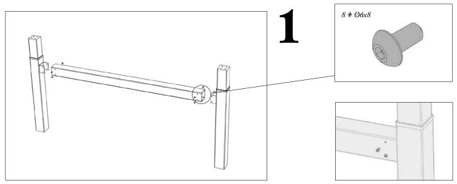
Loosely attach the table legs to the cross bar, then tighten, once the table frame has been fitted (see picture 4).
