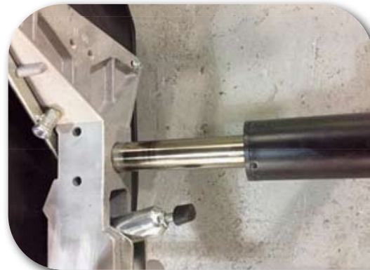
Insert top stem of cylinder into hole at center of chair mechanism
