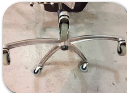
Insert caster stems into sleeves in feet of the star base and you chair is complete!
