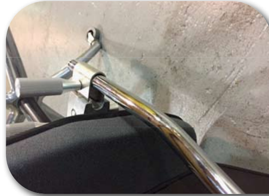
Insert stem of back into back of mechanism attached to the seat. Loosen and tighten hand crank as necessary to insert stem and fix seat back position.
